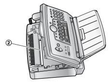
**11** Install the drum and toner unit (①) by holding the tabs.
